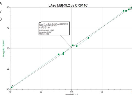
Figure 5: XL2 LAeq dB data for each location vs CR811C LAeq. Fit of 1.001 demonstrates very little difference between instruments.
