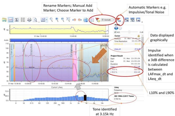
Figure 3: Data Explorer graphical view of Train Station data. Tools for analysis are in the icons along the ribbon. On the graph the LAeq is visible, the peak caused by the train horn is indicated by the pink marker and an impulsive noise is identified. A tone is visible on the 1/3 Octave chart beneath the graph.
