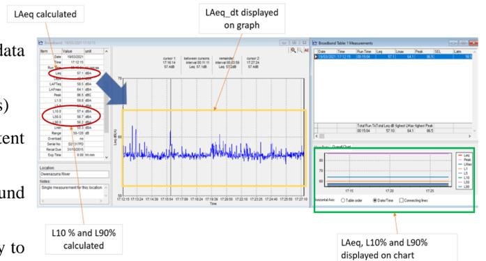
Figure 4: Deaf Deffier3.3 displaying Owenacurra river data. The LAeq, L10% and L90% are shown calculated and displayed on the right-hand chart. The running average (LAeq\_dt) is seen on the graph.
